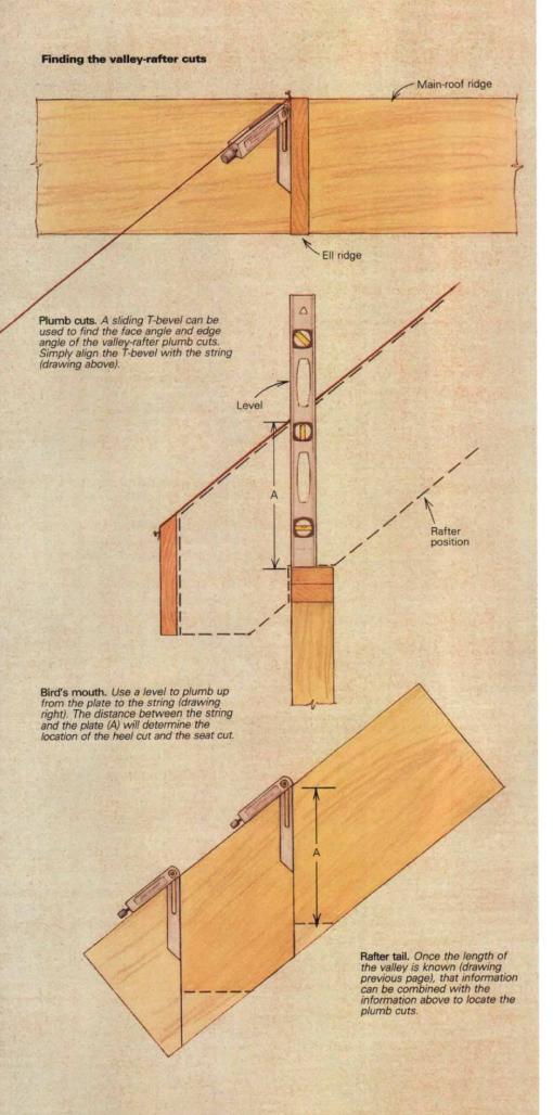
about, especially if the span is long. The string is a convenient guide for constantly checking alignment. Temporary braces may be needed to hold the valley rafter to the line until all the framing is complete.
