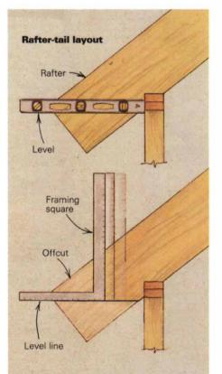
Determining the length and cutting pattern for a common rafter tail on the ell can be done without calculation. Snap a level line on the wall, corresponding to the common rafter level cut on the main roof. Then use a spirit level to transfer this line to the common rafter tail. Slide a framing square along this line until it measures a given distance along the vertical leg; this will be the plumb cut.
